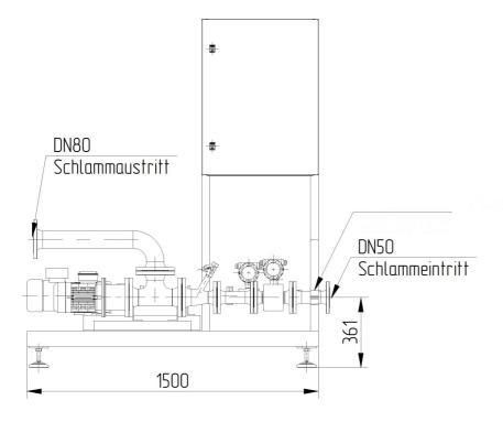
Mechanical structure and arrangement of the components. Illustration as an example, may vary depending on version.
